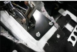
2) Use the provide flange bolts to secure the front of the shifter plate to the floor in the factory locations.
