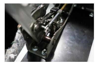
4) Route shifter cable and wiring per your needs. Note in picture below, the shifter is used with the Watson Racing Cobra Jet center stack. Note the notches in the panel for cable and wiring clearance.
